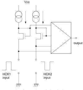
Level conversion equivalent circuit
