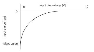
Pull-in current characteristics at the input pin
